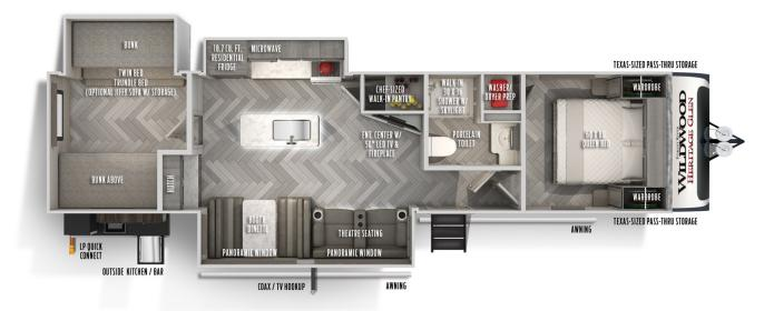
Hitch Weight: 1200 lb. UVW 9088 lb. **CCC** 2312 lb. **Exterior Length:** 38' 6" **Exterior Width: Exterior Height:** 11' 2" 96" Fresh Water: 57.00 gal. **Gray Water:** 78.00 gal. **Black Water:** 30.00 gal.
